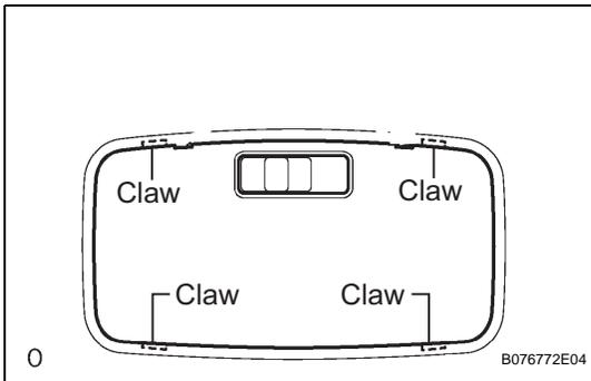
(c) Attach the 4 claws to install the room light lens.
