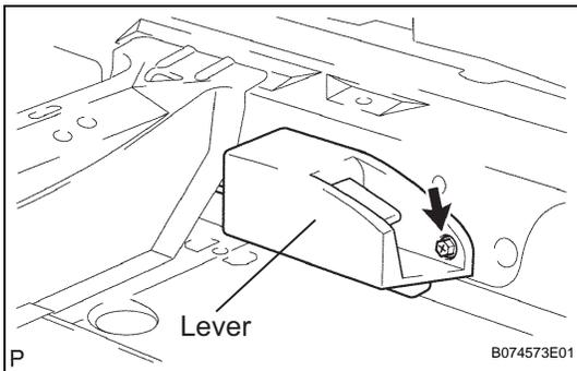
**11. REMOVE FUEL LID LOCK CONTROL CABLE SUB-ASSEMBLY**
