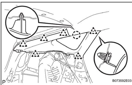
**39. REMOVE ROOF SIDE INNER GARNISH ASSEMBLY LH**
