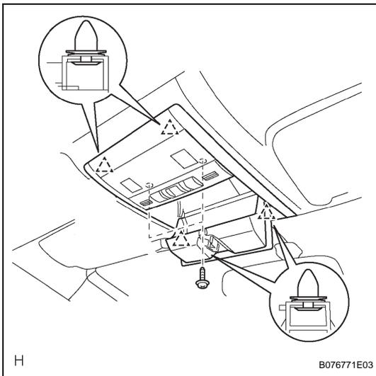
(b) Attach the 4 clips to install the map light.
